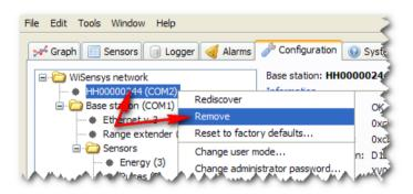
Figure 16: Removing the range extender from the network node
