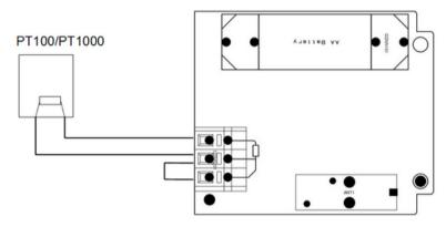
Figure 19: Connecting a 2-wire sensor probe
