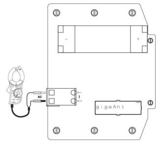
Figure 33: Connecting a battery powered WHT-204AC
