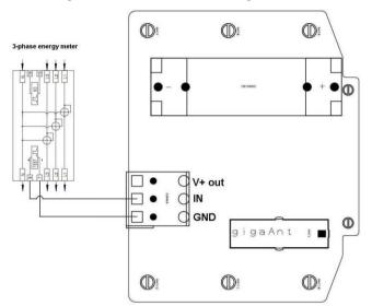
Figure 34: Connecting a WHT-204P to a 3-phase source
