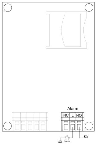
Figure 6: Connecting the alarm relay
