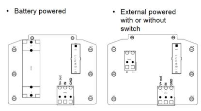
Figure 24: Sensor connections on DLX sensors
