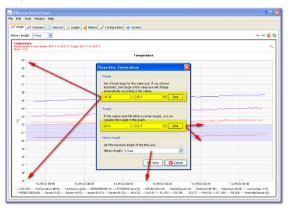
Figure 42: Graph properties dialog, showing a configured range, target and history length
