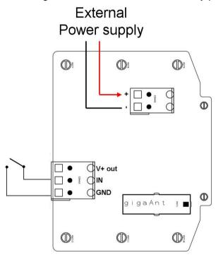
Figure 32: Connecting an externally powered WHT-204C/ct/cc Follow the pairing procedure as described in "Adding sensors to the system".
