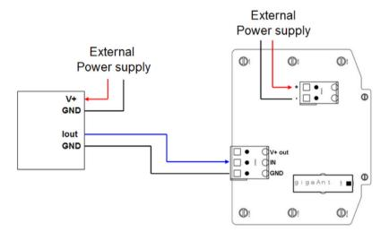
Figure 28: Connecting an externally powered probe to an externally powered WTT-204A sensor
