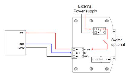
Figure 29: Powering the external probe by the WTT-204A sensor
