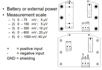
Figure 27: Connections and measuring scales of WHT-204M
