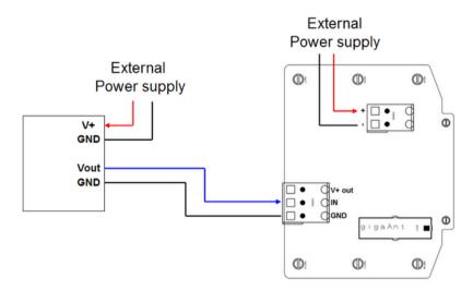
Figure 25: Connecting an externally powered probe to an externally powered WTT-204V30 or WTT-204V4 It is also possible to power the external probe by the WTT-204V30 or WTT-204V4 sensor. See the figure below for the connections.
