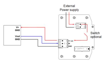
Figure 26: Connecting an external probe to an externally powered WTT-204V30 or WTT-204V4 and powering the external probe by the sensor
